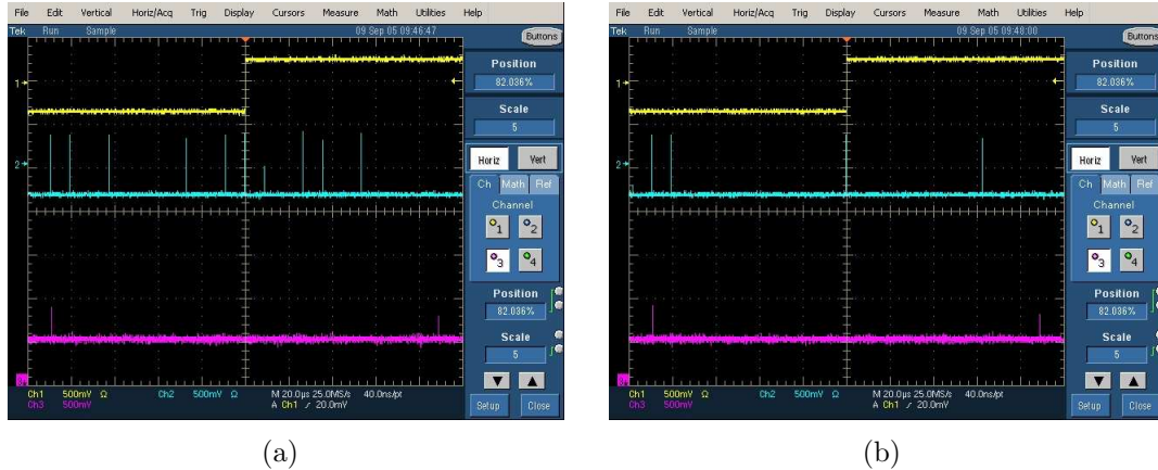
Figure 2.7: Two examples of the APVe asserting ERROR when an orbit BC0 from the TCS-9U coincides with a L1 trigger. The magenta trace shows the BC0 strobe, the cyan trace represents L1As and the yellow trace represents a READY \rightarrow ERROR transition. Note the missing BC0 when it coincides with a L1 trigger.
